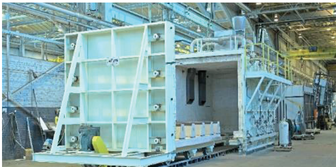
Car Bottom Furnace
